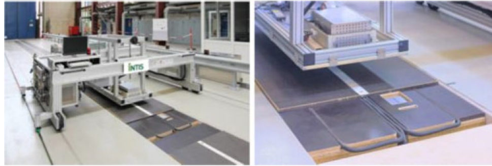
Fig. 23. Test frame for a pick-up (left) and double U-type power supply rail (right) used in the test center [90].
