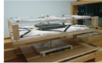
(c) Reduced ferrite DD
