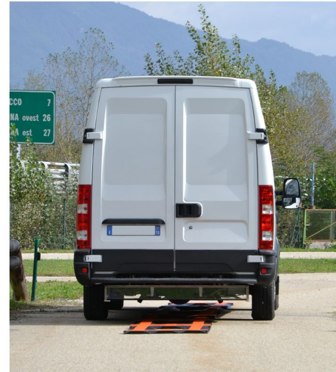
Fig. 12: Back of the vehicle during the CWD operation. Under the vehicle plane is visible the receiving structure mounted.
