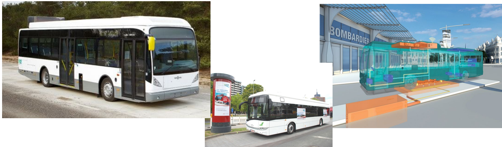
Bus: Dynamic trials lowered pads at controlled height, Stationary lowered for 100-200kW
