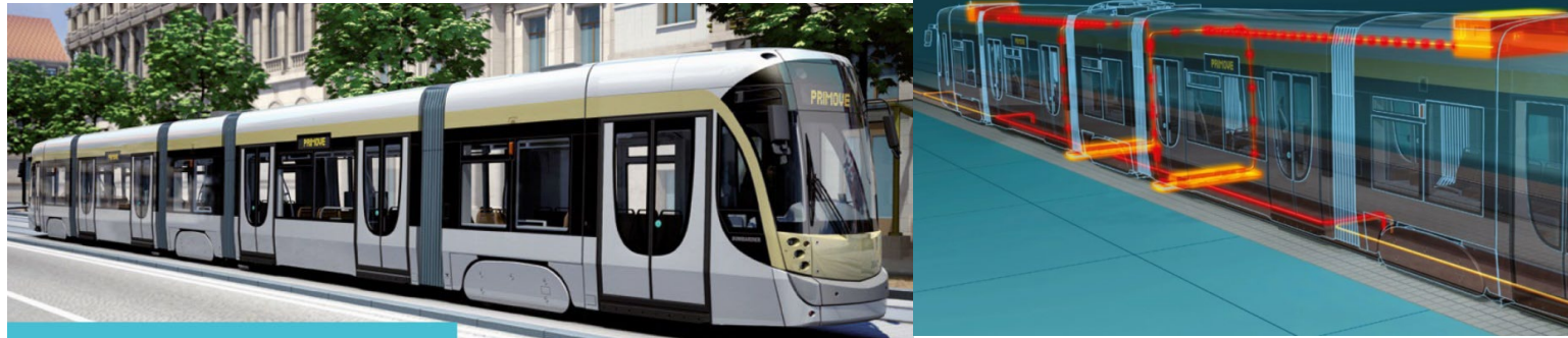
Light Rail: Continuous 270kW power, buried cables replaces catenaries
