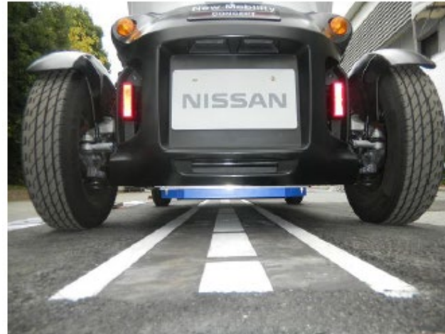
Figure18: Photograph of the receiver coil installed at the rear of the test EV
