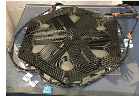
3 phase 120° rotated DDs ORNL.
